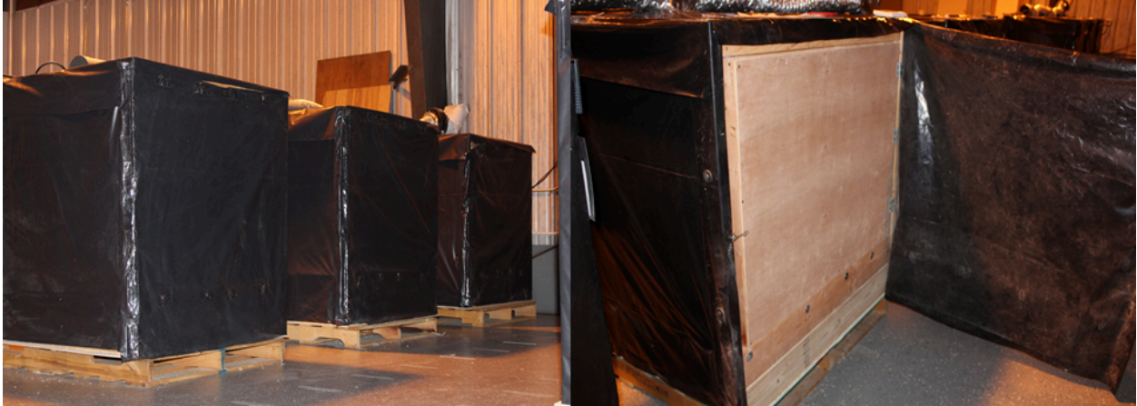
Figure 1 Figure 1. Individual “tent” housing structures constructed of wooden boxes, placed on pallets that were covered with black, opaque plastic to create an individually controlled lighting environment. (A) Three separate tent housing enclosures that included one treatment per tent (approximately 16-18 young pullets/tent). (B) A tent enclosure with the outside plastic opened to show the wooden door that was used for accessing the bird housing area.
